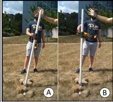
Figure 1 (left): Free body diagram and equations. Figure 2 (right): Illustrative example of the tail effect. The initial pendulum angle of 22 degrees (A) from the vertical position was corrected to 2 degrees (B) after activating the tail.
